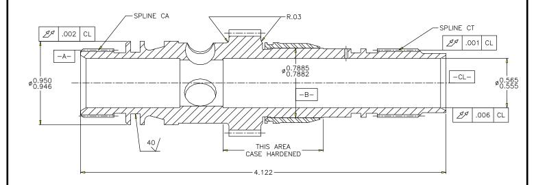
SPLINES CA AND CT HAVE 0.7500" PITCH DIAMETERS.
