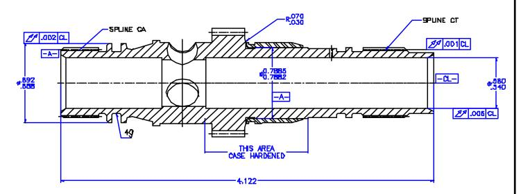
SPLINES CA AND CT HAVE 0.7500" PITCH DIAMETERS.
